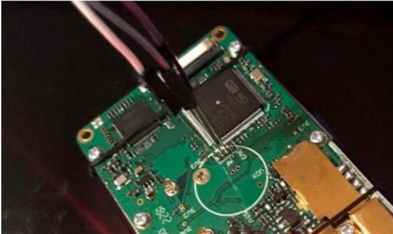
10. While powering up the ST Link program, power the radio in firmware update mode by pressing the PTT and top red button while powering on. The red LED will flash.
