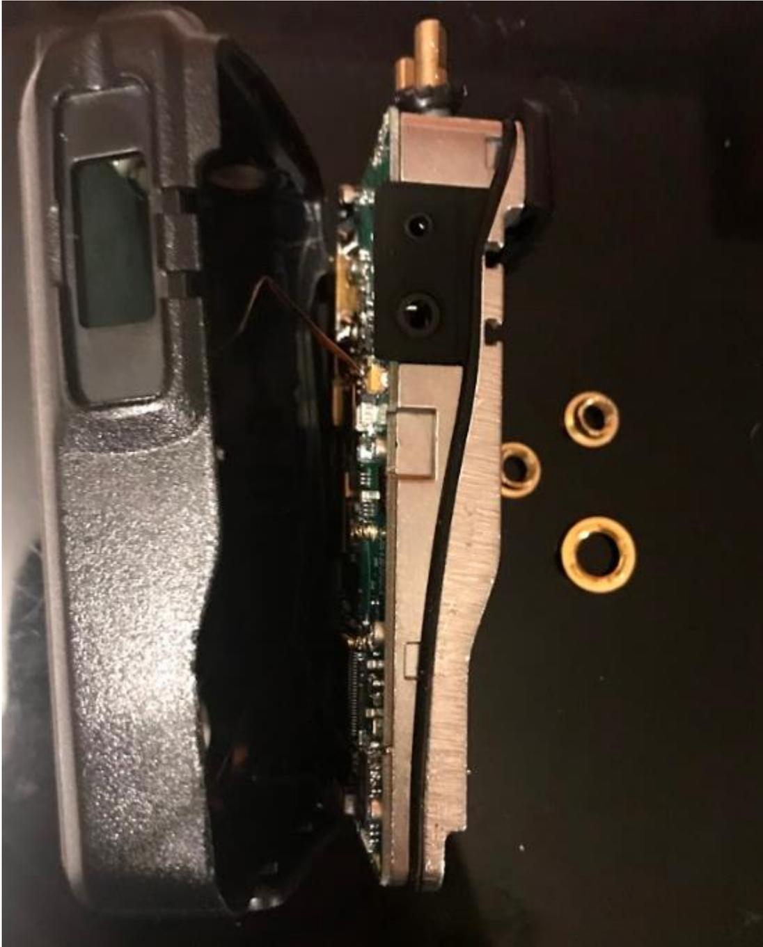
7. Making sure to not damage speaker/mic and screen ribbons remove the ribbons from the connectors, after pushing the clips up with a thin screwdriver. The speaker ribbon has already been removed in the photo below.
